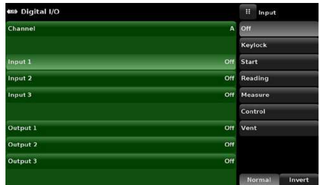
Figure 6.4.11-B - Digital Input Assignment
