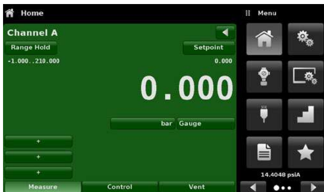
Figure 6.4.1-B – Single Channel Display
