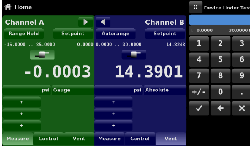
Figure 8.9.2.3-C - DUT pressure for purge sequence
