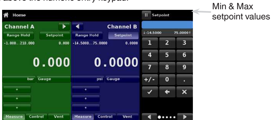
Figure 6.4.1.2.1 - Numeric Keypad Setpoint Entry
