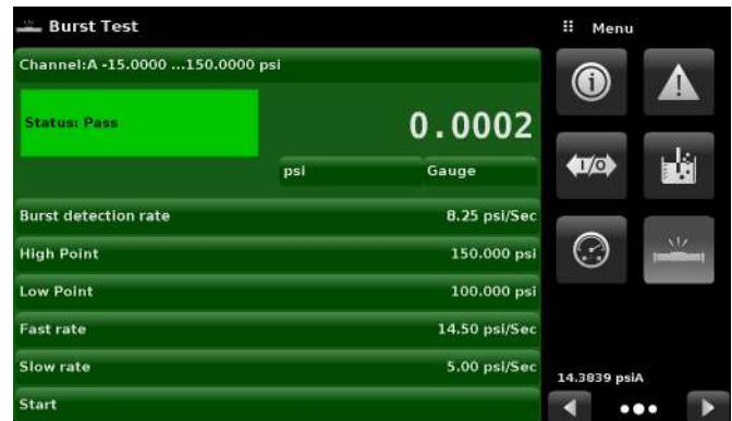
Figure 6.4.14-C - Burst Test Complete (No Burst)
