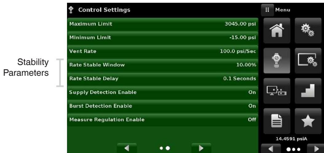
Figure - 6.4.3.9 Rate Stability Parameters
