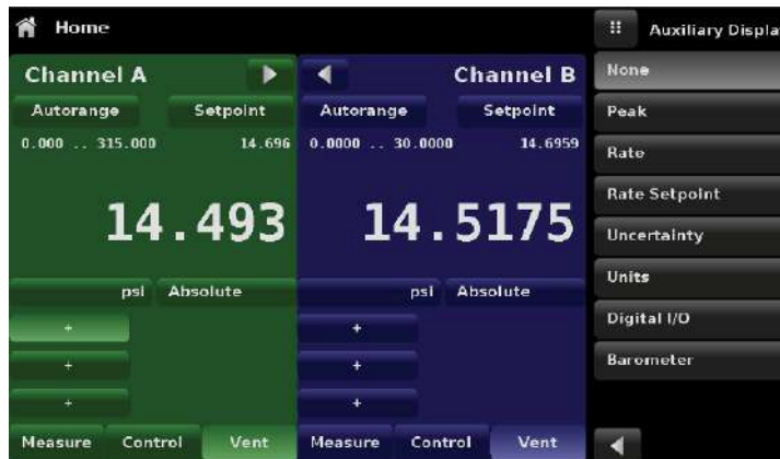
Figure 6.4.1.5-B - Auxiliary Display Selection
