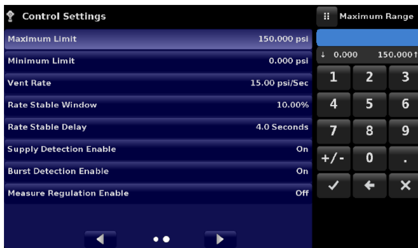
Figure 6.4.3.7 - Control Limit Setting
