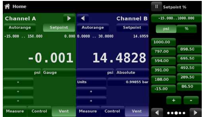
Figure 6.4.1.2.3-B - DUT Pressure Value Entry
