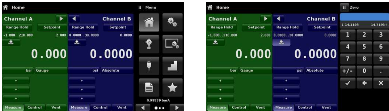
Figure 6.4.1.6 - Zero Button, Gauge - Absolute
