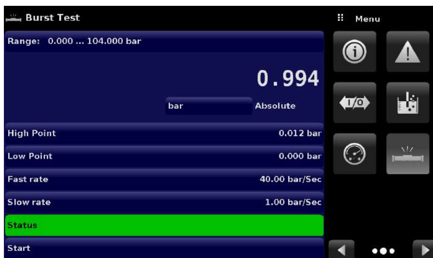
Figure 6.4.14-B Burst Test Complete (No Burst)
