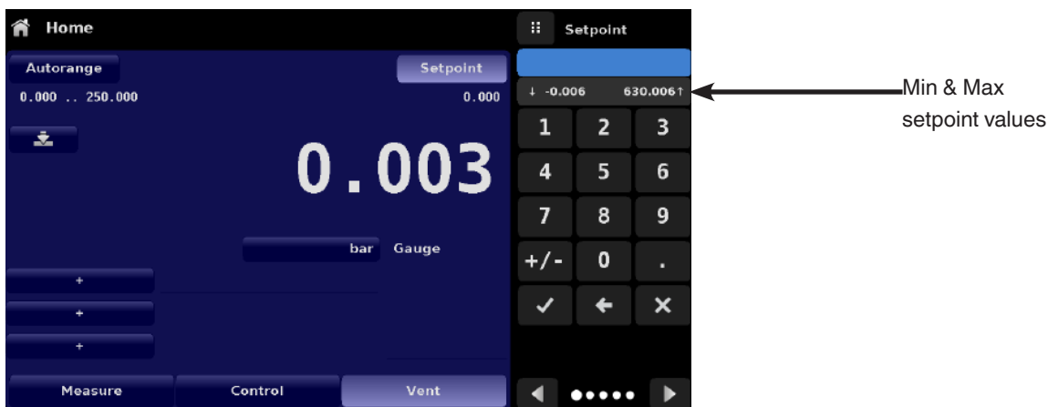
Figure 6.4.1.2.1 Numeric Keypad Setpoint Entry
