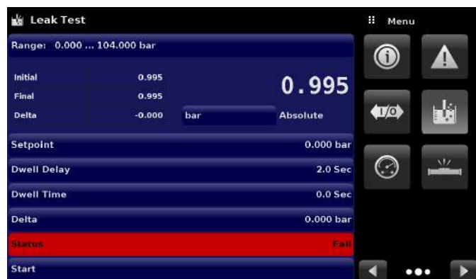
Figure 6.4.12-A Leak Test Fail (left) and Pass (right)
